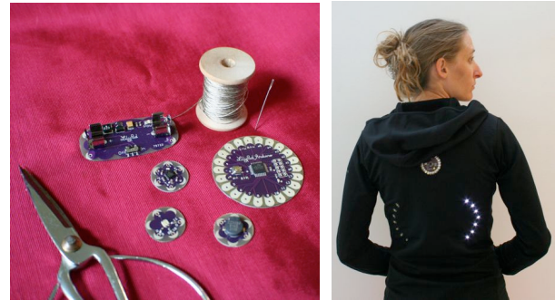
Figure 1. Components of the commercially available LilyPad kit and a sample construction, a turn signal biking jacket.
